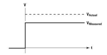
Figure 2. Resistive loading reduces the amplitude of the measured signal without altering the shape.
