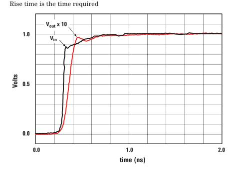
Figure 12. A probe's minimum rise-time can affect your measurements.
