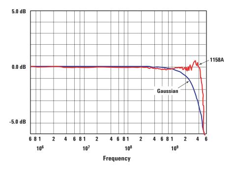
Figure 13. Comparison of Gaussian transmitted response and the steep roll-off of the Agilent 1158A probe.
