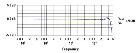
Figure 8. (Top) Frequency response of  $V_{in}$  and  $V_{out}$  of the Agilent 1158A, 4 GHz probe. (Bottom) Since the frequency response of  $V_{out}$  closely tracks  $V_{in'}$  the transmitted response of the probe remains flat throughout the 4 GHz bandwidth of the probe.
