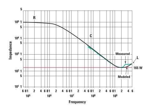
Figure 4. Increasing frequency changes the input impedance of the Agilent 1158A probe.
